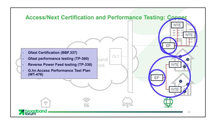
BBF has a full suite of certification and performance test programs for copper transmission . BBF.337 has gone through several iterations certifying Gfast functionality, and its companion TP-380 specifies performance testing. We also have tests for the Reverse Power Feeding, which is frequently used to power nodes out at the distribution point. Finally, we're developing a plan to test performance for GHNA access technology.
