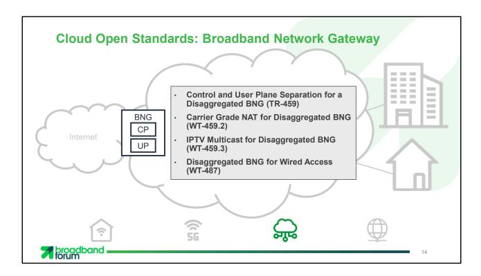
Quite a few nodes in the broadband network can benefit from disaggregation. As we virtualize the network, many of the functions that used to be implemented as dedicated boxes are being virtualized and disaggregated.
