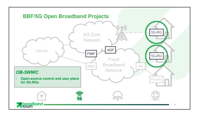
On the Open Broadband front, the OB-5WWC project is creating an open-source reference design for the 5G-enabled residential gateway.
