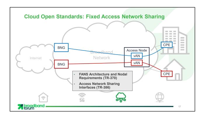
One final topic within Cloud is Fixed Access Network Sharing, or FANS. Some regulators have required incumbent broadband operators to open their networks at the physical layer to multiple service providers. The way we facilitate that is by specifying multiple virtual instances of the Access Node. Each virtual instance can be managed and configured by a different network operator. The virtual networks are isolated so that each operator only sees, and controls, their own part of the network.
