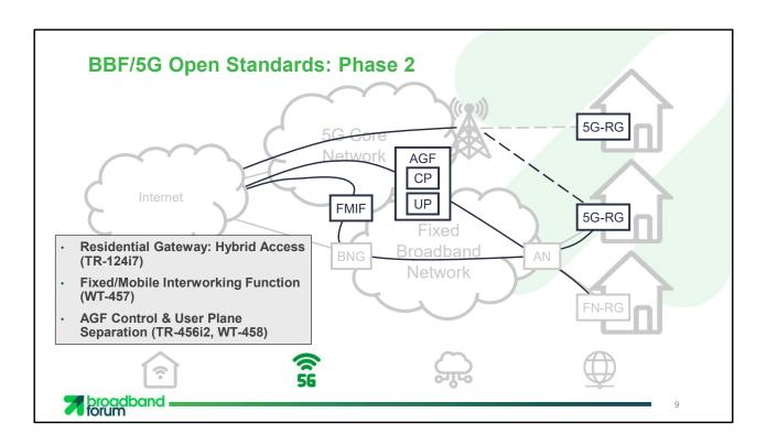
For Phase 2 of BBF's 5G work, the first item of business is hybrid access. We've added 5G access requirements to the residential gateway, so it can be used either for fixed wireless access or wired access in 5G convergence. Why not both? This has resiliency applications, and it also provides additional bandwidth for certain scenarios.
