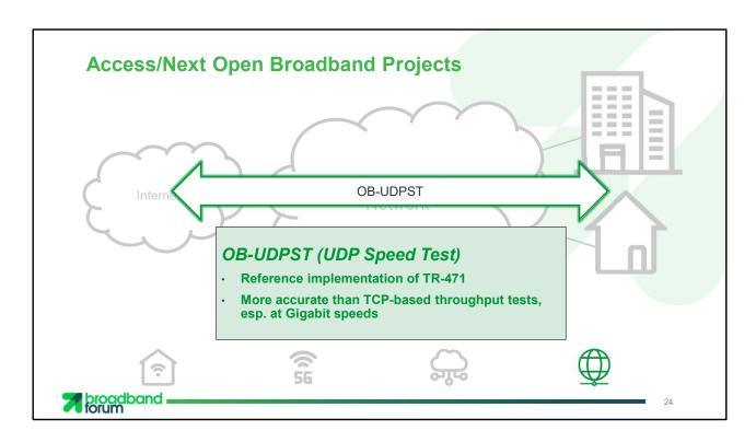
UDP capacity measurement brings us to our last Open Broadband project, which is a reference implementation of a UDP based speedtest. Like all of our Open Broadband projects the releases for this project are available on GitHub.
