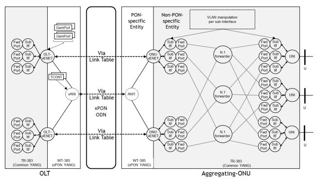
Figure 6 – Ethernet Service Model (Combined-NE mode with Aggregating ONU)
