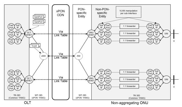
Figure 7 – Ethernet Service Model (Combined-NE mode with Non-aggregating ONU)
